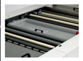
Rollers and brushes are mounted with snap lock bearings, so they can be instantly replaced without tools or the need to re-calibrate pressure.
